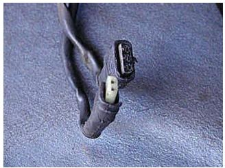
Inspect the electrical connections. Using the contact cleaner and other cleaning supplies, thoroughly clean the electrical connectors. The boots around the connectors are rubber. After cleaning them, applying Gummi-Pflege will help condition them.
