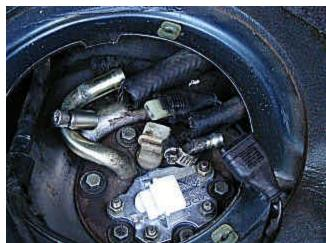
String the electrical connectors in place (the smaller electrical connector will not slide under the smaller fuel hose easily after its connected).
