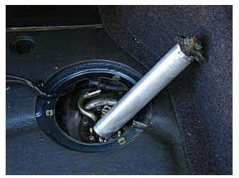
Slowly pull the fuel sending unit up. The sending unit will be full of fuel, and the space for the fuel to drain is small. Just let the sending unit sit as shown until the fuel stops leaking from the bottom. Set the sending unit aside on something that will absorb any remaining fuel that spills.
