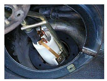
Put the pre-pump gasket in place, roughly lining up the holes.
