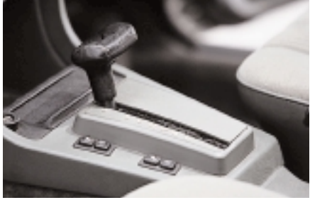
Four-speed ZF automatic gearboxes on later cars need regular fluid changes for long life.
